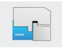
Keeps ice for days\* The labyrinth seal prevents any heat from making its way into the interior
